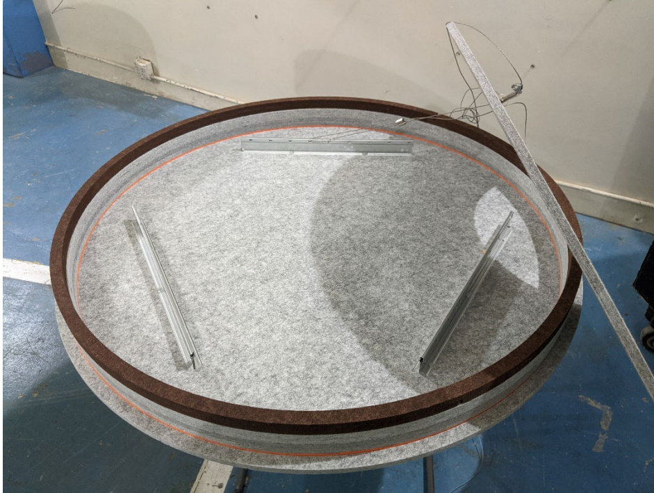
Figure 3 – Detail of added felt strip (brown felt ring) installed to individual baffle; baffle top temporarily removed
